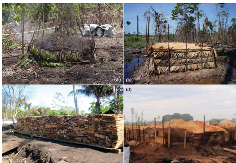
Figure 2. (a) Rural earth mound kiln. (b) Rural sawdust covered artisanal kiln. Sawdust is derived from nearby sawmills or transported down rivers from the city. (c) Urban kiln in construction. (d) Urban kiln in carbonisation.
