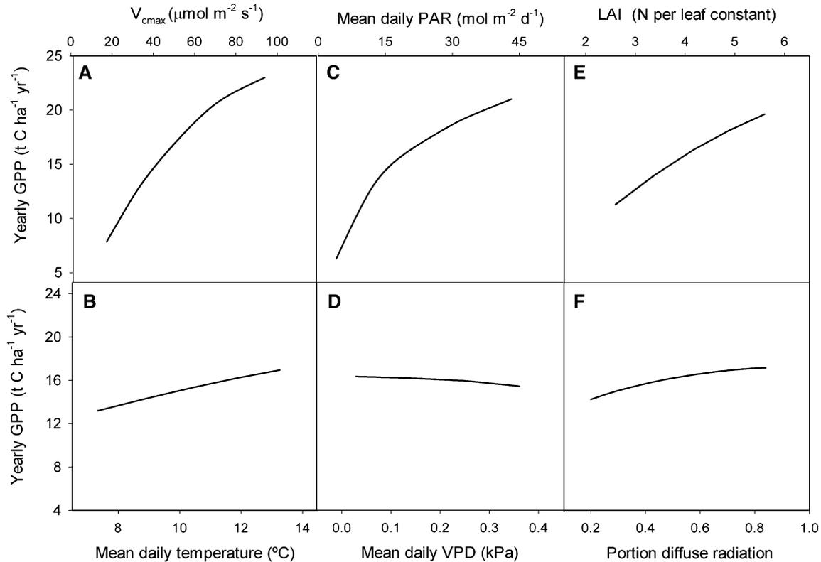
**Figure 5.** Results from the one-dimensional sensitivity analyses for six important factors over their observed range controlling annual TCMF GPP. Note that for panel **A**, both  $V_{cmax}$  and  $J_{max}$  were changed concurrently, whereas only  $V_{cmax}$ , and only the value of the top layer of the canopy is listed on the *X-axis*.
