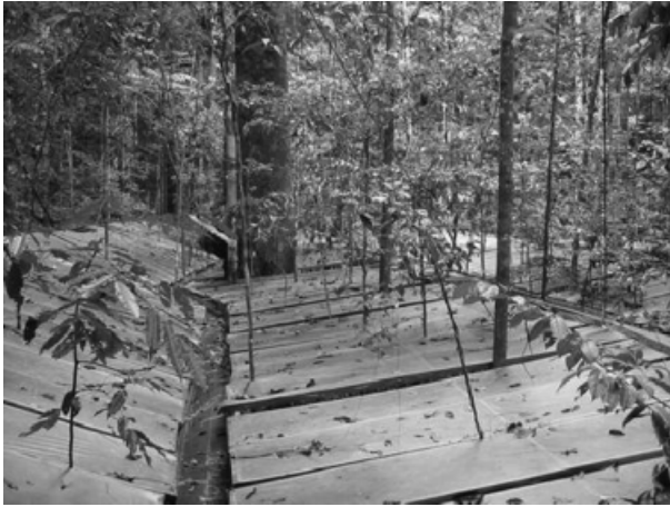
Fig. 1 Throughfall exclusion installation at Caxiuanã forest. One hectare (100 m × 100 m) of plastic panels draining into aqueducts intercepts incoming rain and drains it away from the soil, causing an artificial drought. The panels cover ~80% of the ground area and were in place throughout the whole duration of the experiment, with the exception of the 4–21 November 2002, when they were removed.
